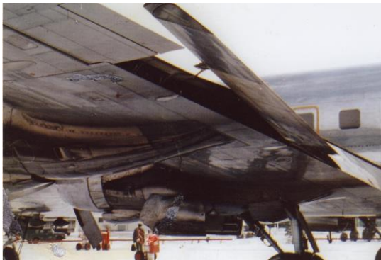
The flaps of N90781 at Osan after the 23 December 68 emergency landing (photos taken by Ed Fleck, kindly submitted by Jesse Walton)
