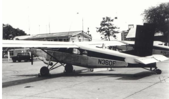
PC-6C N360F with an Air America cowcatcher, that is a deflector bar in front of the tail wheel; the photo was probably taken at Vientiane in the early seventies (UTD/Anthony/F9)
