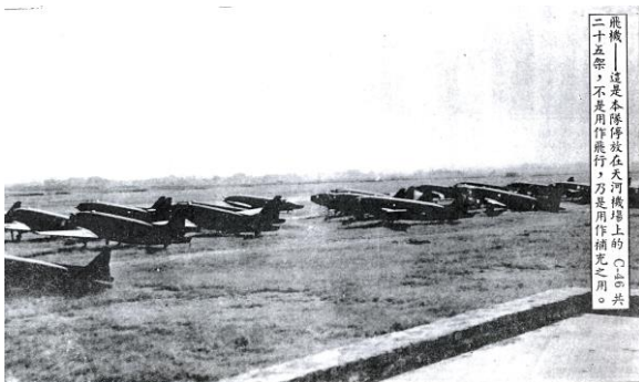
SALVAGE PLANES—Hulks of 25 C-46s owned by CAT stand on Tien Ho airfield in varying degrees of cannibalization. For months CAT’s salvage crews have been removing equipment and parts from them to keep the rest of CAT’s fleet in the air.
