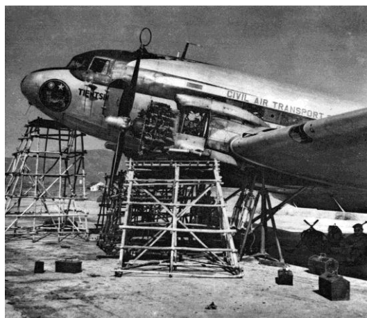
CAT C-47 “Tientsin” being maintained (UTD/Burridge/ photo no. 1-AB1-1-PB19)
