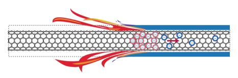
**Figure 1** A chemically driven thermal wave (shown in red) generates thermally excited electrons in a thermopower wave; its propagation to the cold (blue) end of the nanotube can be harvested as electrical energy. Figure courtesy of Ali E. Aliev.
